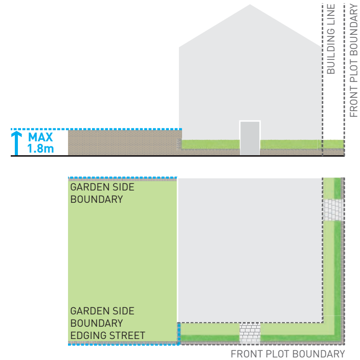
DP8.6 Fig1 Side Boundary / Corner Treatments
